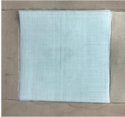
Figure 1. Stacks in the cavity of Teflon films before pressing.
