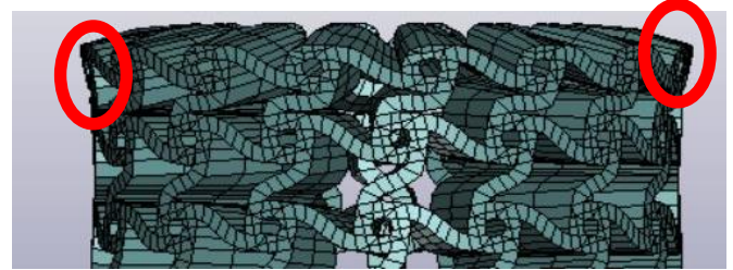
Fig. 10. Scheme of tetrachiral structure with expanding layer.
